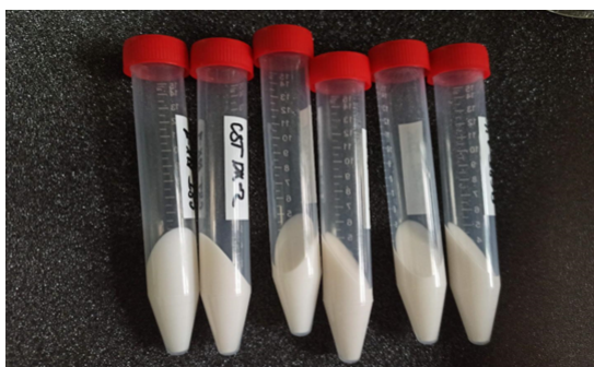
Fig. 2. Day and Night cream formulations after the centrifugation test after the period of 18 months storage (from the left to the right: DC-1, DC-2, NC-1, NC-2, NC-control and DC-control, respectively).
